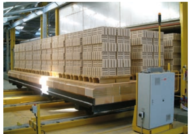
Kiln car exiting a tunnel kiln.
