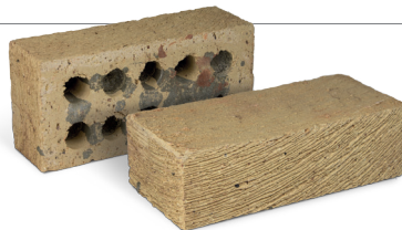
Heavily textured BD.1.3 created from a standard perforated brick using the fill & face method. Texture created using epoxy.
