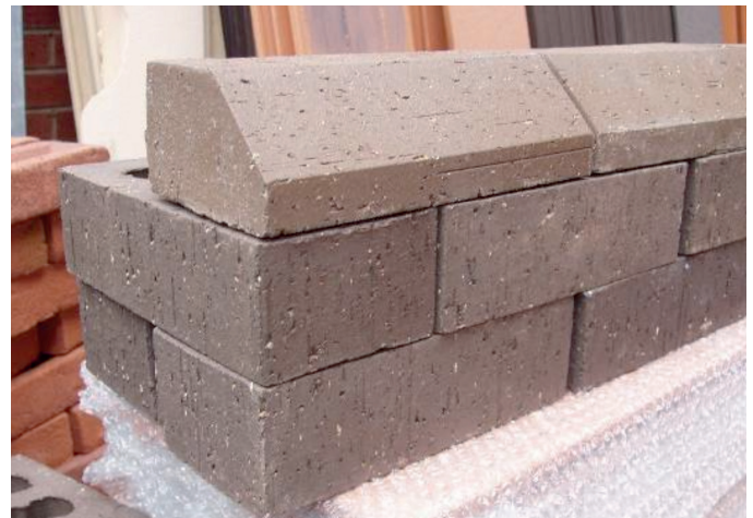
Due to different extrusion processes, the drag wire marks on the plinth bricks run horizontal whilst the standard bricks are vertical.
