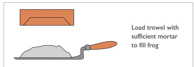
To lay bricks with frogs down and filled, the trowel must be loaded with sufficient mortar and brick and trowel lowered into position.
