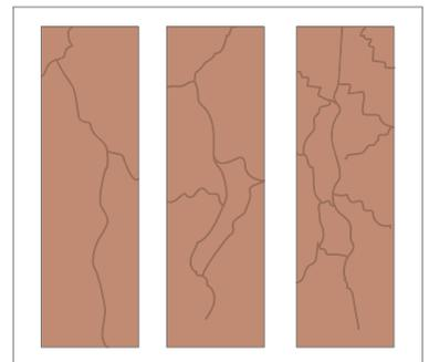
The crazing is undetectable to the eye whilst the bricks remain dry prior to use or whilst very wet.
