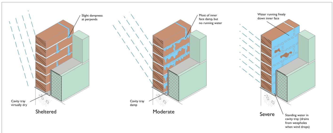
During long periods of wind-driven rainfall, the brickwork becomes saturated directing excess water down the outer face. Mortar, often being more porous than the masonry unit or prone to hairline cracking, will absorb large volumes of water which then enter the cavity.
